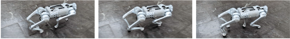
Fig. 1: High-speed Running Without Reward Shaping. We train a policy to run at high speeds with just two reward terms: velocity tracking and energy minimization. Furthermore, our approach automatically and adaptively balances these two terms online during training. This is due to Extrinsic-Intrinsic Policy Optimization (EIPO), a constrained policy optimization algorithm that strictly prioritizes the velocity-tracking task performance while treating energy minimization as an intrinsic reward.
